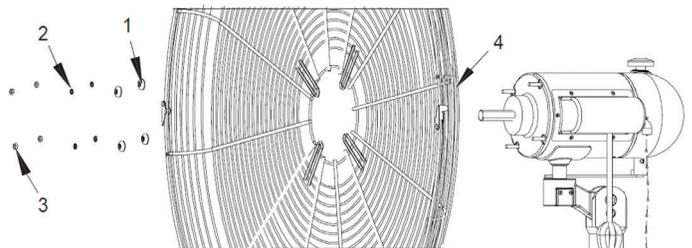
6. Attach the blade (2) to the shaft on the motor and secure them together using two screws (1).
