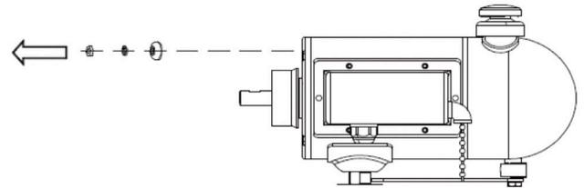
5. Attach the rear guard (4) to the screws found on the motor and secure them together using four bowl washers (1), four spring washers (2), and four nuts (3) from step 4.
