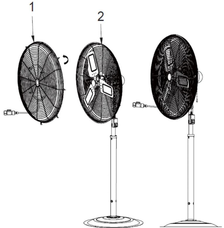
8. Secure the assembly on the front and rear guard by tightening the screw (1) and nut (2) on the bottom of them.
