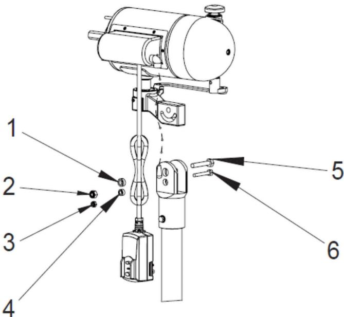
4. Remove four sets of hexagonal nuts, spring washers, and big washers from the motor. Save them for step 5.
