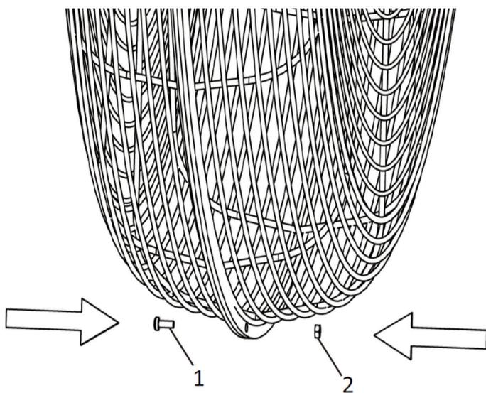
9. Connect the misting switch (1) to the water pipe (2) and tighten it. Turn the switch (open) to open the misting function. Turn the switch (close) to close the misting function.
