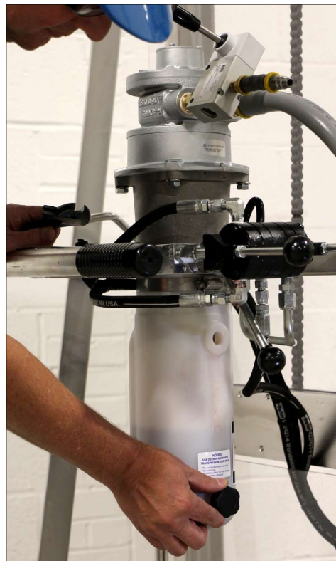
Remove BLACK breather from storage position
