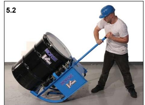
6. With drum in horizontal position, it is now ready to be moved to desired location to begin drum rolling operation.
