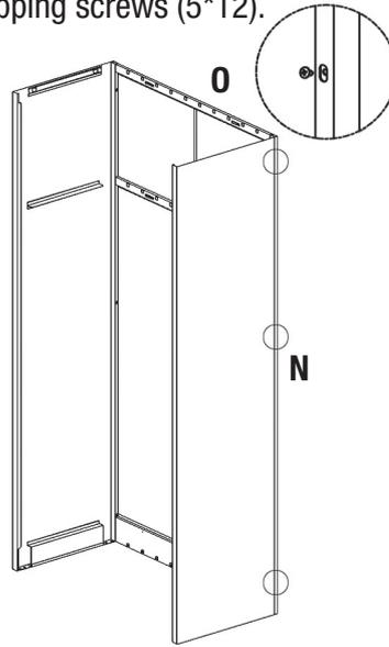
(3) Open the door and clip the door frame to the side plates.
