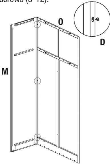
(2) Bolt the right side plate and back plate together with 3 self-tapping screws (5\*12).
