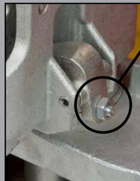
Use proper set screw and lock nut adjustment located on the side of the pump. This feature was designed to ease the pallet truck adjustment. Tools required are: flat screwdriver and a 14mm wrench.
