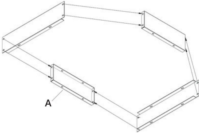
**1.** Begin by bolting together all four base panels (A). Using 8 nuts and bolts, with the nuts on the inside of the base (*Figure 1*). Tighten bolts with a 3/8" nut driver.
