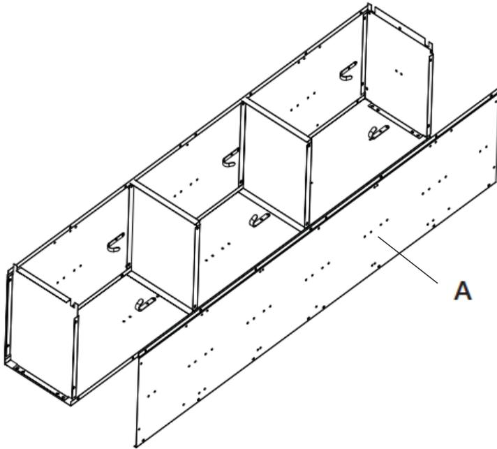
5. Bolt the right side panel (A) with the angles, going around the back panel. Bolt the side to the top, bottom and shelf. Also, bolt the third coat hook to the right side panel (*Figure 3*).
