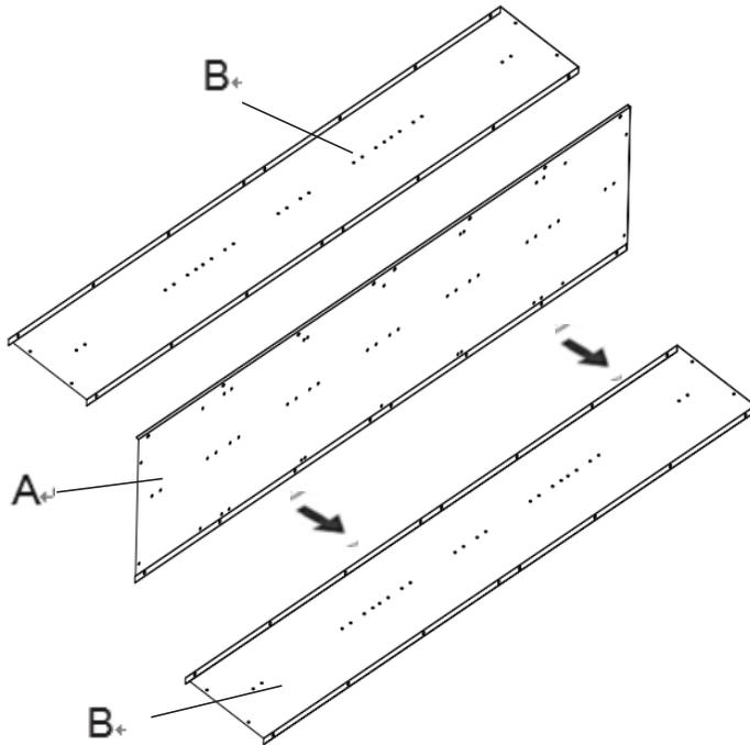
Only tighten bolts with a 3/8" nut driver once the locker is completely assembled.
